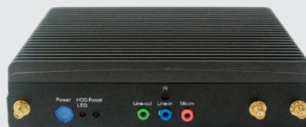
Figure 1. Chassis for Compact, Fanless Version
