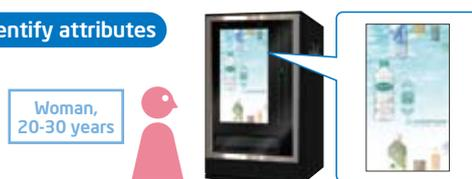
The camera in Intel Digital Vending determines the gender and age bracket of the customer and automatically recommends products that match the target. Where items are displayed is also adjusted based on the customer's height.
