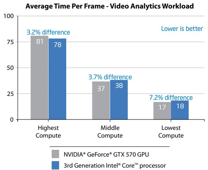
Figure 3. Graphics Performance Comparison between the NVIDIA\* GeForce\* GTX 570 GPU and the 3rd Generation Intel® Core™ Processor GPU
